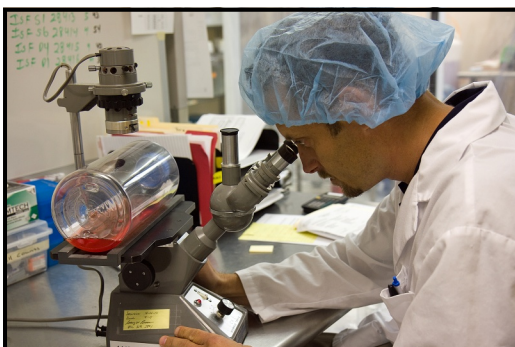
Figure 4. Examining the cells using an inverted microscope for lysis or cytopathic effects (CPE) to determine if the influenza virus has grown.
